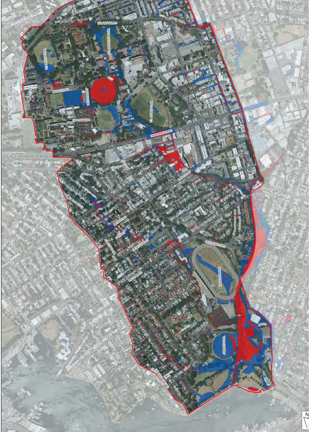
FIGURE 16 HAZARD CATEGORIES 2% AEP DESIGN FLOOD EVENT
